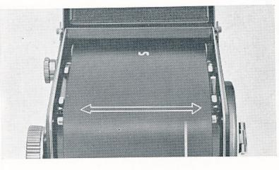
6 Wind on until the "Start" mark on the film leader aligns with the red "Start" marks on the camera.
