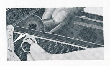
To minimize the trouble in loading your next film, it is advisable to take out the empty spool from the lower film chamber and to set it in the upper chamber immediately after unloading the exposed film.
