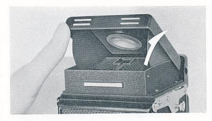
Set the Focusing Hood upright by lifting it up all the way. The Focusing Screen feature eight red lines which facilitate picture composition.
