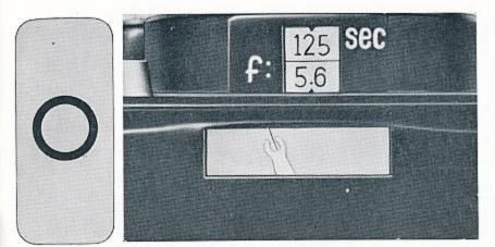
When the yellow follower needle (Y) perfectly coin-cided with the meter pointer(I), it signifies that your YASHICA 12 is set for correct exposure. The proper combination of the shutter speed and aperture is shown in the Shutter Speed and Aperture Indicator Windows.
