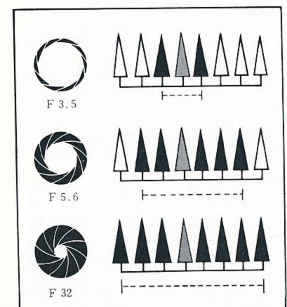
The depth of field is the range in the foreground and background over which all objects appear acceptably sharp when the camera is focused on a given subject. The extent of the depth of field varies with the aperture of the lens and the camera-to-subject distance.
