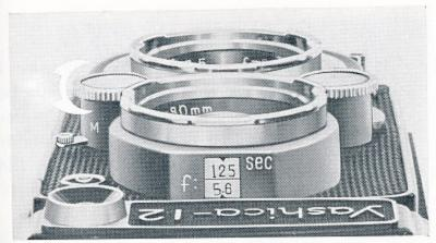
In case the correct combination of shutter speed and aperture is 1/250 sec. and F8, turn the Aperture Control Dial and set the lens aperture to F 5.6 when using a Y2 filter.
