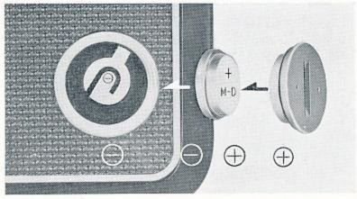
Place the mercury battery in the Battery Compartment, make sure the (-) side faces inside. The lid will fail to close if the polarity of the battery is reversed. One replacement of a mercury battery provides sufficient power to work the meter for a period of about two years under normal Use. However, it is advisable to check the battery once
