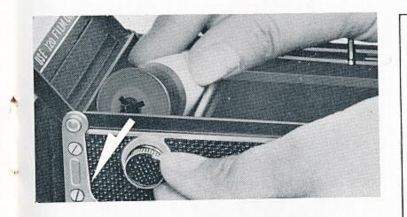
Pull out the Upper Spool Holder Knob and take out the exposed film from the film chamber. Paste the seal to prevent recoiling and wrap the film in light-proof paper.
