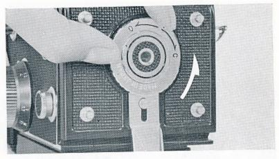
The entire length of the film has been exposed when the Exposure Counter registers the figure "12". Another turn of the Crank-handle will bring out the ⊚ mark in the window, but continue winding until the Crank-handle turns freely.
